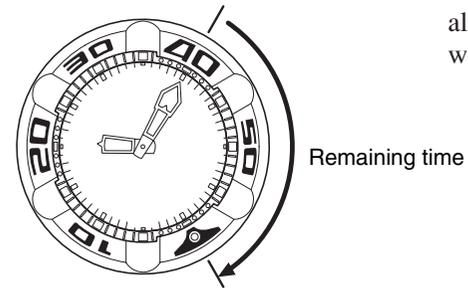
\* The remaining time can be determined by aligning the ▼ mark on the rotating bezel with the target time.
