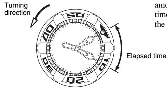
\* Align the ▼ mark on the rotating bezel with the minute hand. After a certain amount of time has elapsed, the elapsed time can be determined from the scale on the rotating bezel.
